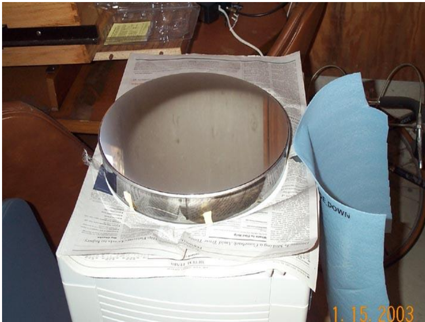
The Mirror Grounded, Polished, Parabolized, Coated
